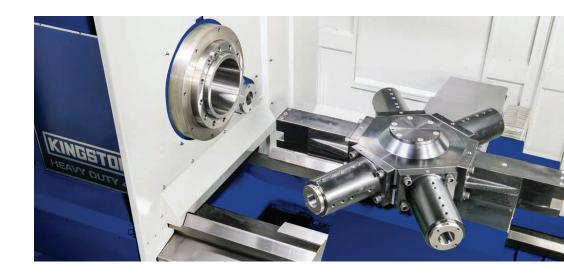
Kingston's CK Chucker model uses its big features to combine powerful heavy-duty cuts with high accuracy. The 4-speed headstock and robust spindle construction are built for high turning torque (9,000 N-m at low speeds), while the heavily ribbed one-piece casting and brawny 28-inch wide 2 V-way bed provide extreme rigidity when cutting large-diameter workpieces.
