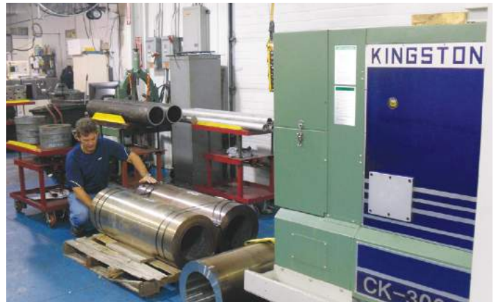
Sam Wilcoxon inspects incoming 17-4 stainless steel castings for roll bodies, each weighing around 2,000 lbs before machining. The ID will be bored out approximately 8" resulting in a finished ID of 11-1/2".
