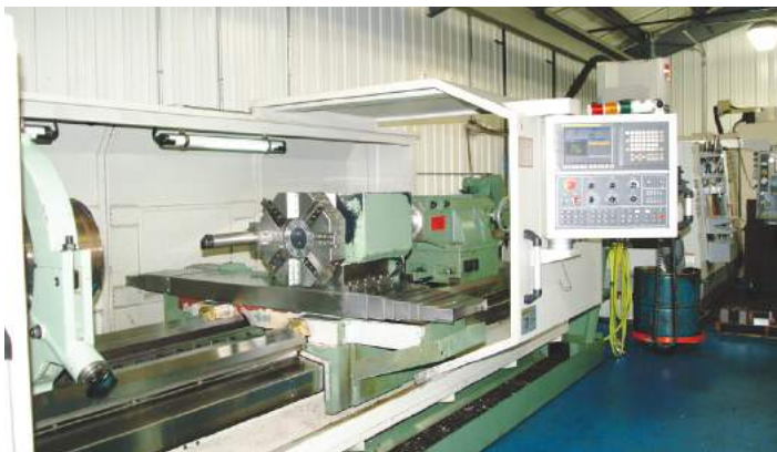
Kingston CK 3000 CNC lathe set up with a roll body ready for machining.
