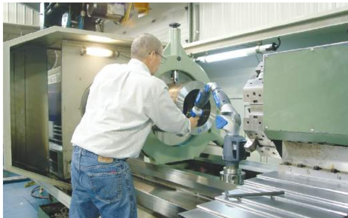
After machining, Mike Moore inspects the ID dimensions of a roll body with a FARO Gage. There is ample room inside the Kingston CK 3000 for inspection with the portable CMM arm while the workpiece remains on the machine.
