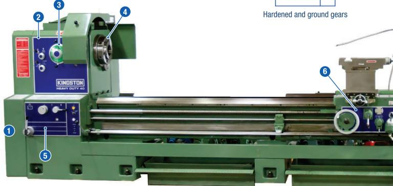
5 Feed Gearbox coarse thread cutting up to 8" lead.
