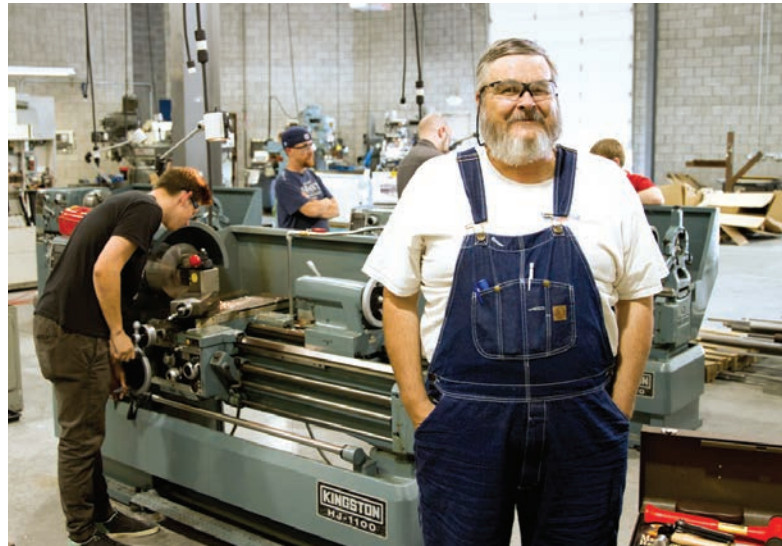
Instructor Barry Maxfield developed MATC's Machine Tool Technology program, which uses Kingston HJ 1100 engine lathes for manual machine training.
